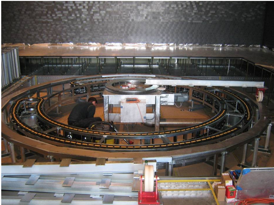
Figures: Principle of energy chain
